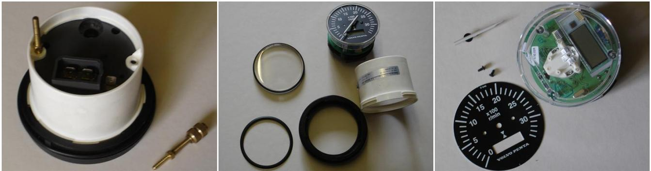
The old LCD display can be prised out with a blade under the edge - the ribbon cable 'can' be pulled out but it is better to try and lever up the sides of the white terminal block to release (5,6,7):
